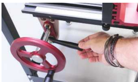
▲ Positions can be easily locked using the cam lever
